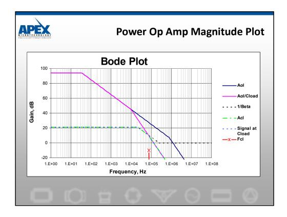
In any composite amplifier, make sure the power output stage is stable first. Any of the techniques we learned earlier can be used.
