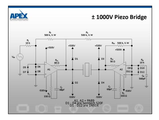
Piezo users appear to never have enough voltage. As soon as it was introduced the PA89 found its way into bridge circuits to drive piezos at +/1100V and beyond.
