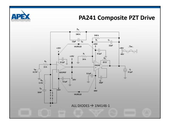
This circuit is included as an example in Power Design.xls. It is different from most power op amps in that current limit from positive side to negative side does not match well at all.
