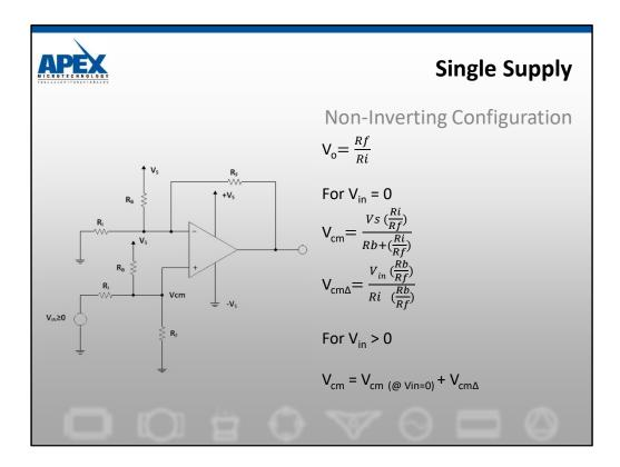
This configuration can easiest be viewed as a differential amplifier with an offset voltage summed in on both + and - input nodes. With this arrangement of resistors the transfer function is: Vout = Rf/Ri Vin.
