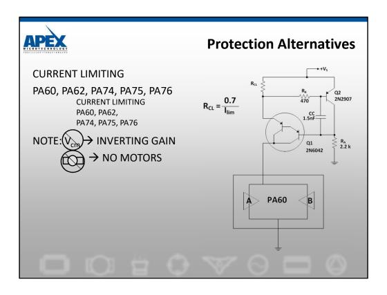
This handy circuit can be used with the PA60 series amplifiers in a single supply application to provide external current limit with minimum components.
