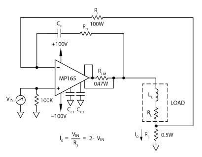
Floating Load Voltage-to-Current Conversion Circuit
