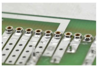
Part number MS11 consists of a carrier strip of 30 cage jacks. The strip can easily be cut to any desired number of cage jacks. These are mounted directly in a print circuit board. After soldering, the carrier is pulled off the cage jacks. Use a spacer between the PCB and the heatsink to avoid short circuits.
