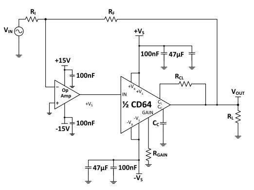
Figure 1: Typical Connection (Composite Configuration)
