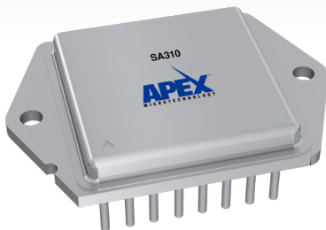
Fig 7. The smallest member of the Apache family, the SA310CR, is packaged as a Power DIP device to allow it to deliver 30 A of continuous current per switch, and up to 80 A peak current.
